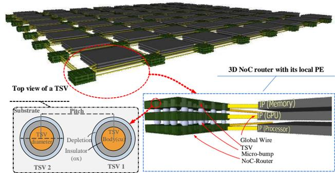
Fig. 1. Stacked 2D planar, vertically interconnected by TSVs in 3D integration technology
