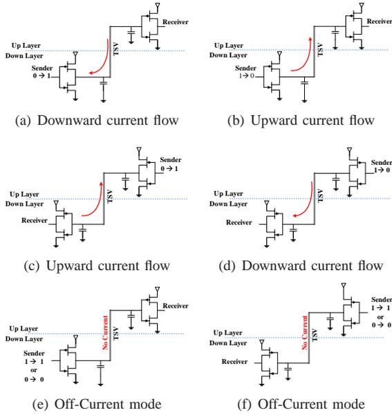
Fig. 3. Current flow direction in TSV.
