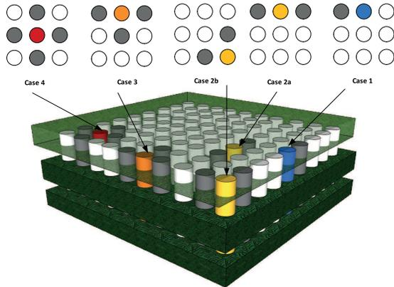
Fig. 4. Different TSV patterns leading to inductive coupling
