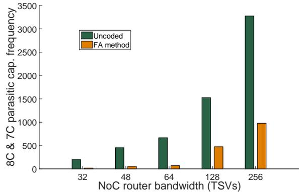
Figure 9: Number of 7C/8C for random data bit patterns in small mesh of TSVs
