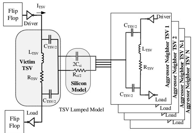
Figure 1: The block diagram of the induced capacitive coupling on each TSV based on physical parameters
