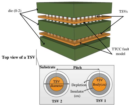
(a) Fault model location in IC simulator
