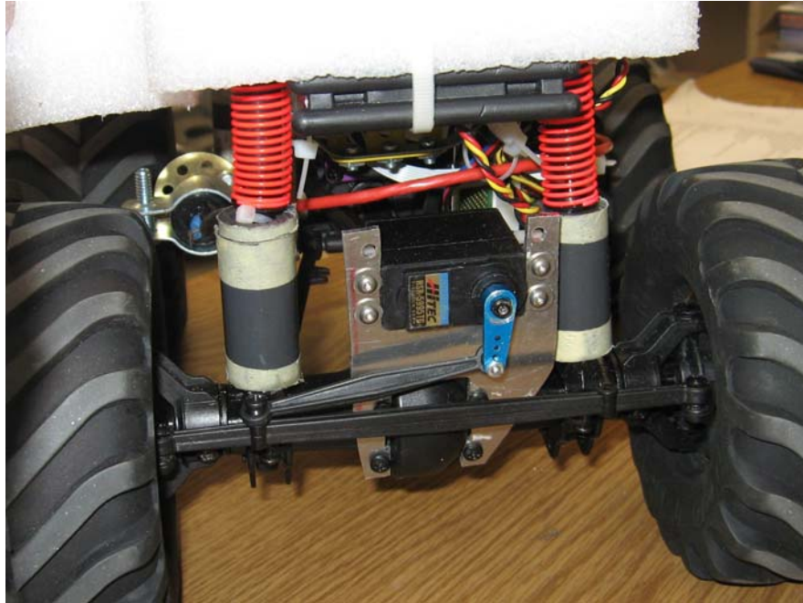
Figure 3: Modified high torque steering servo and linkage.
