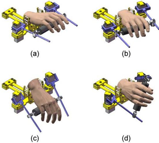
Fig. 2. 3D renderings of CRAMER showing (a) the neutral position, (b) ulnar deviation of the wrist, (c) wrist flexion, and (d) forearm supination. The orientations of the guide rods determine the wrist orientation.
