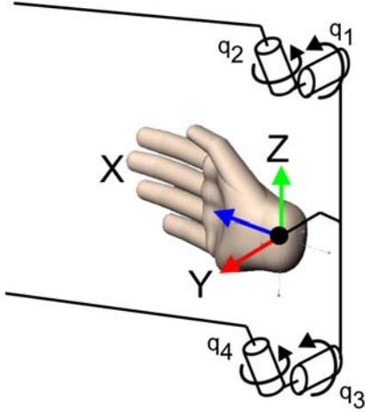
Fig. 4. Simplified schematic of how the motors configure the guide rods. The hand is in its home position.
