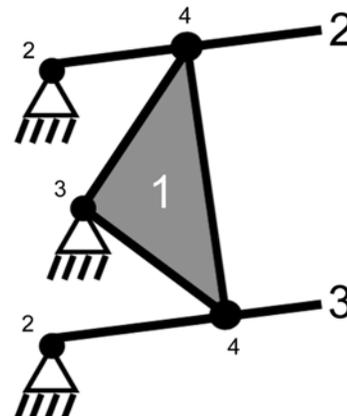
Fig. 3. Simplified schematic of CRAMER with its links numbered and joints labeled by mobility. The ground makes up the fourth link.
