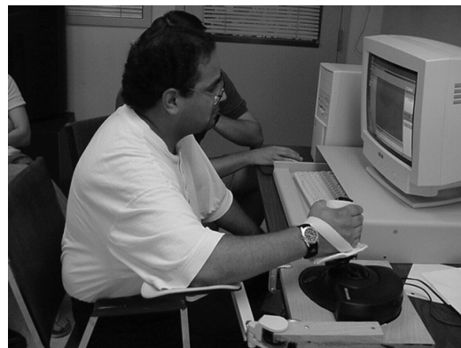
Figure 1: Prototype web-based, force feedback telerehabilitator (“Java Therapy”)
