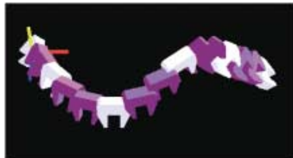
Figure 2: The same end-effector trajectory but interpolated using double quaternion coordinates of six key-frames.
