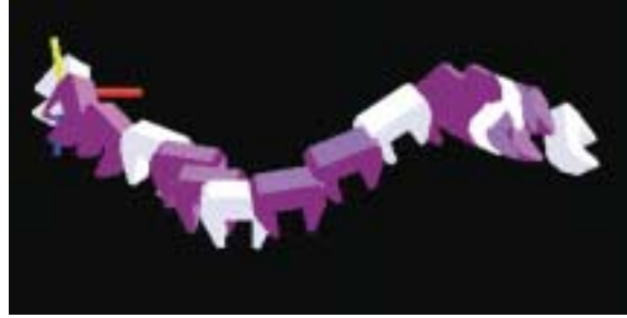
Figure 1: The end-effector trajectory that interpolates the dual quaternion coordinates of six key-frames.
